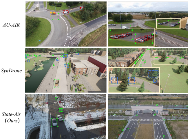
Figure 4: Annotation comparison among State-Air, AU-AIR, and SynDrone. Green: labels given by the datasets; Yellow: revision of incorrect labels; Red: missed labels; Blue: negative labels.
